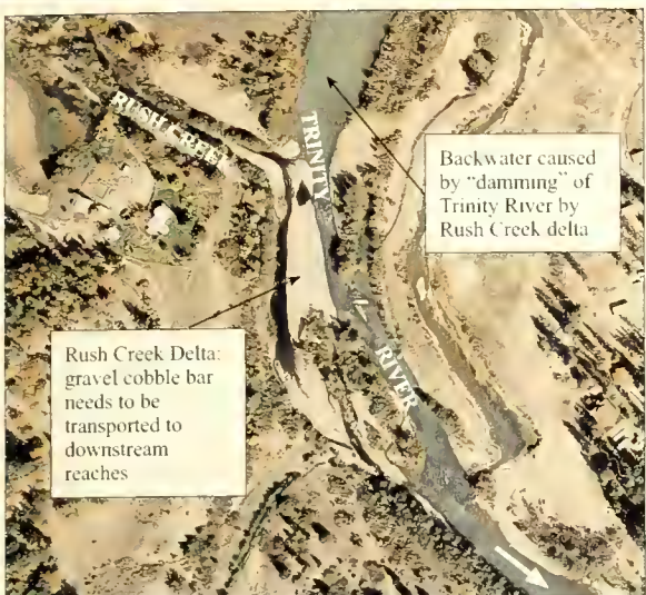
Air photo of Rush Creek Delta showing local sediment accumulation and upstream backwater "lake"
